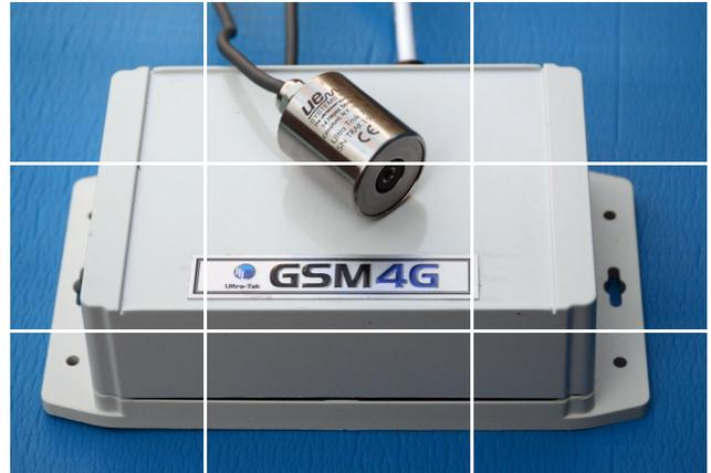
The **Ultra-Tek GSM4G™** unit uses a standard phone sim card and a **UE Systems Ultra-Trak 750™** Ultrasound sensor providing 24/7 real time information. The trigger points can be remotely set and altered by sending an SMS instruction to the unit. The user can dial in at any time to see real time information on the performance of the equipment. Each unit is PIN protected and multiple phones can dial in to see live data, if PIN is included.
